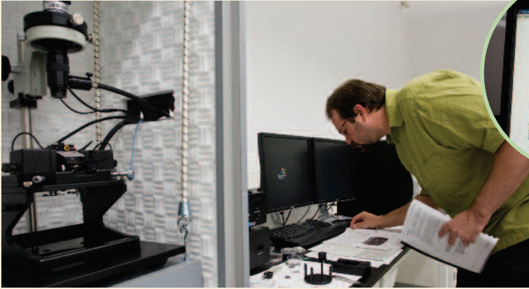
Dr. Garrett Clayton, Assistant Professor, conducts research in the Image-based Controls Lab that is focused on using images to calibrate, model, and control dynamic systems. The system pictured is an atomic force microscope, which can be used for extremely high resolution surface imaging.
